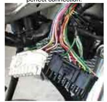
Insulate the soldered connection, and also the bare ends of the snipped wires with insulation tape. I use 3M insulation tape which is excellent for the job.
