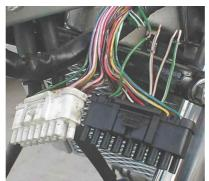
Snip the LtGr/R, Gr/P & Gr/W wires approximately 60mm from the black connector, and remove 5mm of insulation to expose the copper wires inside.
