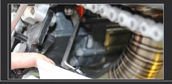
**5)** The rear right stay (with M6 insert) should be secured to the step kit as shown. Just finger tight at this stage.
