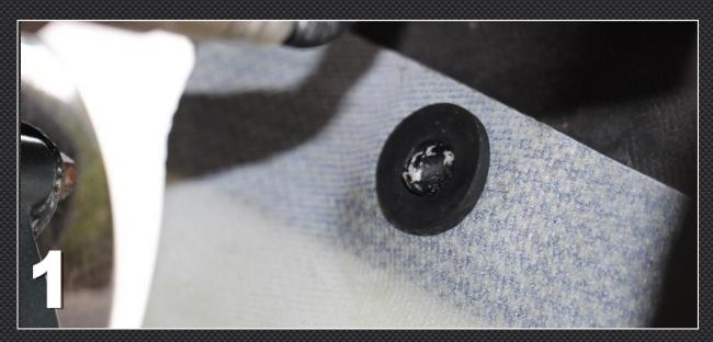
**2)** If not already fitted prior to shipping, fit the drain hole bung to the hole in the Belly-Pan
