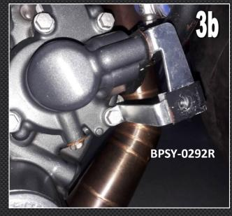
**4)** Attach the lower left rear stay as shown. The M8 bolt on the frame should be screwed through, and then the stay fitted and nipped up with the nyloc nut. Do not fully tighten at this stage.
