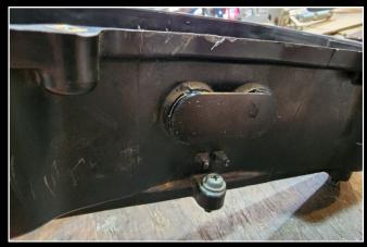
The last things left to deal with are the vacuum hoses to the front intact tracts. We need to block these off to avoid sucking air.
