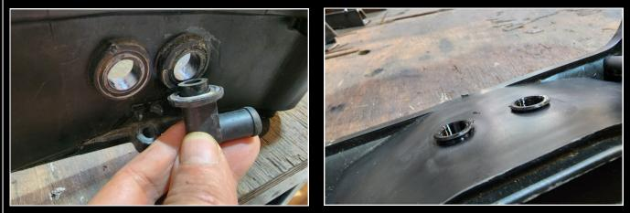
With the spigots removed, blank off the holes using the bung provided.
