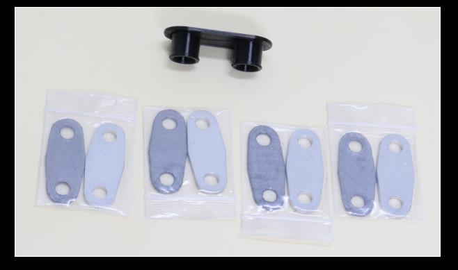
These blanking plates are used to blank off the PAIR Valve holes into the exhaust ports after removal of the complete PAIR valve system.
