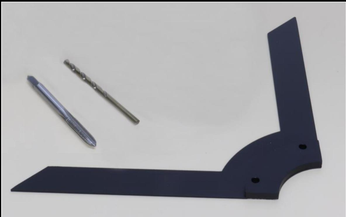
Mounting the BPGF-0009 fuel tank and TYLY-0305 upper/mirror stay on the Honda VFR750F RC36-2 requires that you drill and tap two M6 holes in the headstock area.
