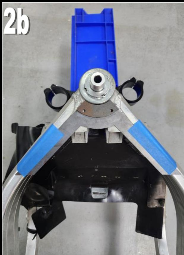
**3)** For a sanity check, mark though the holes with a pen and then remove the jig.
