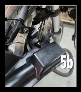
6) Now fit the M4 bolt and plastic washer to the middle mounting point.
