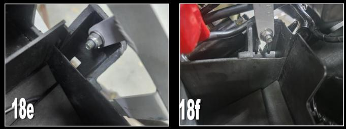
Check that the heat shield mounting tab lines up with the lower right subframe mounting bolt.
