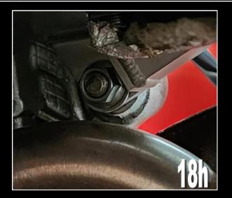
The rubber block on the heat shield should rest on the lower spar of the subframe to assist in damping vibrations. Check that there is no interference of the heat shield with the cylinder head or exhaust headers
