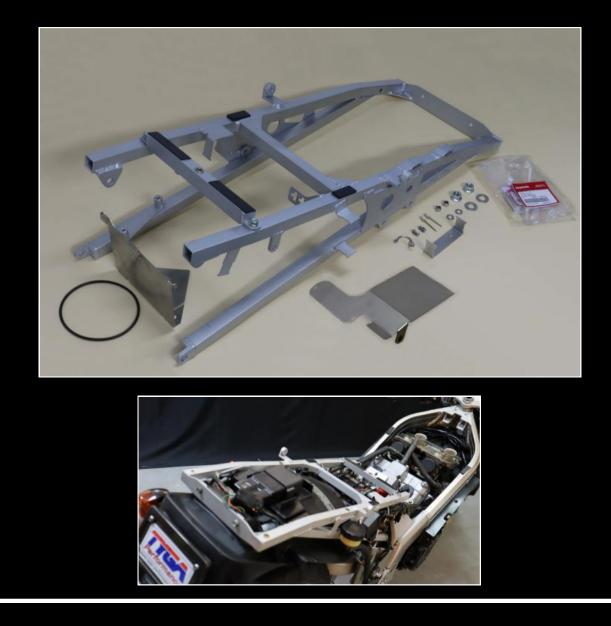
Fitting the TYGA TYLY-0314 subframe is not too difficult. If you managed to remove the standard subframe with ease then the fitting of the TYGA subframe is almost a reversal of that procedure, as we have tried to keep all the components in close to their original position.
