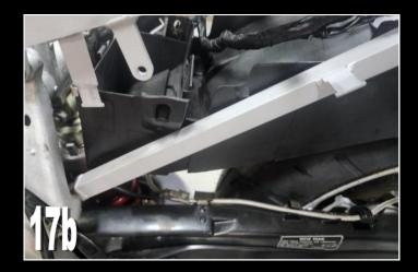
Once in, lift the front into position on the tabs and fit in the original shouldered bolts to retain the undertray in position.
