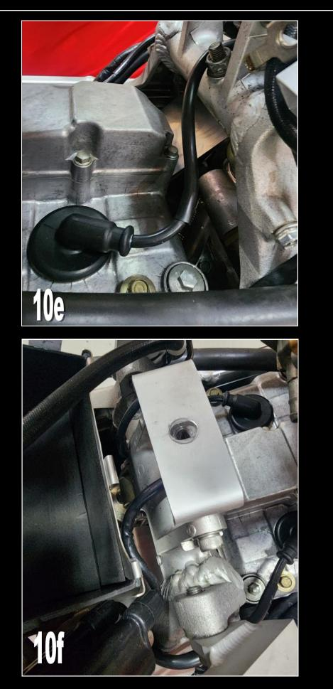
Do not fully tighten the coils up at this stage in case they need a bit of a moving around later.
