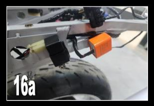
Feed the relay wires through the gaps in the subframe as shown and connect to the main harness. Then they can be tucked out of the way in between the spars. Once the undertray is fitted this will look nice and tidy but can still be accessed if necessary.
