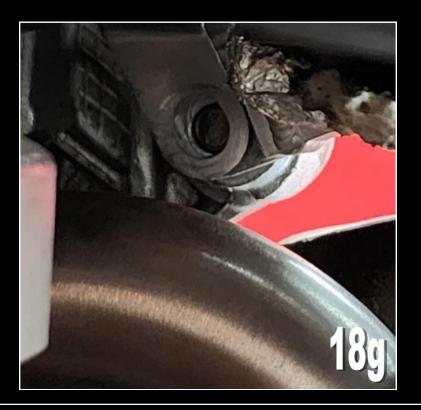
Fit the washer and M10 bolt and tighten.
