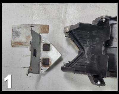
2) Fit the TYLY-0328 Heat shield together with TYLY-0314W battery Plate onto the battery box on the undertray.
