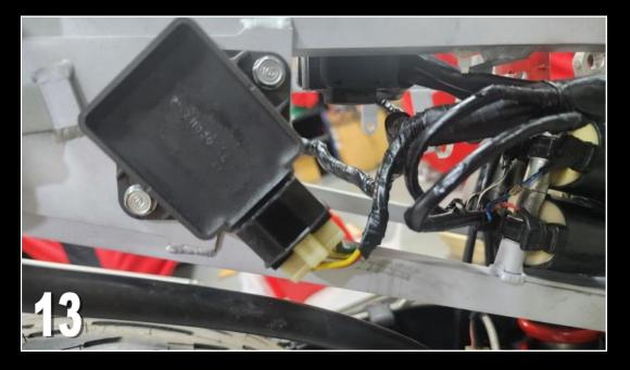
14) Plug the starter relay onto the tabs. Note that all the all the wires are running on the outside of the undertray mounting stay at this point.
