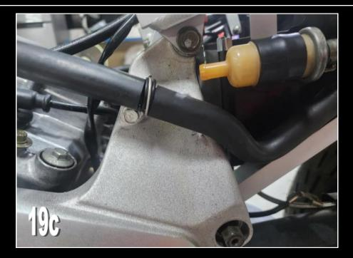
20) Now you can bring the side stand switch and speedo drive module (electronic type) connector up into position. And also the fuel pump connector.Plug them all in neatly to the connector holder.
