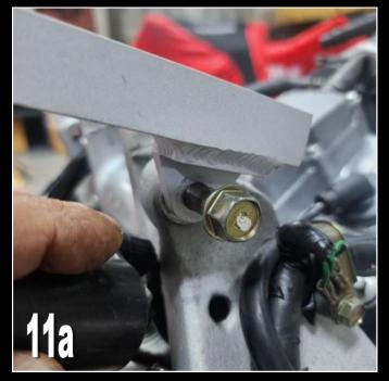
Now is a good time to tighten up a few things. Tighten the two upper mounts and the lower left mount. Loosely tighten the lower right mount as we will later be attaching the heat shield to this point.
