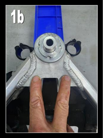
2) Offer up the jig and locate the radius at the front concentric and touching the cover on the preload nut. Take a note of the position of the rearward 'wings' and locate them onto the edge of the frame taking care to make sure that the position is the same left and right.
