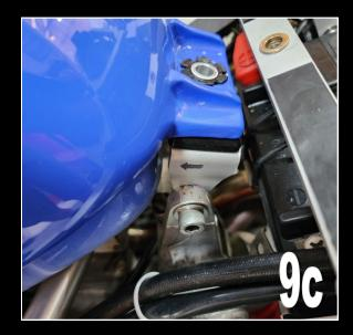
And then fit the M6 bolts (included with TYLY-0305) to the front mount and the M8 bolt (included with TYBP-0006) to the rear mount. Check the rotation of the rear mount to make sure that the stay is parallel. If not perfectly parallel, then the stay can still be rotated a little as it is not 100% tight yet. Adjust to parallel if necessary.
