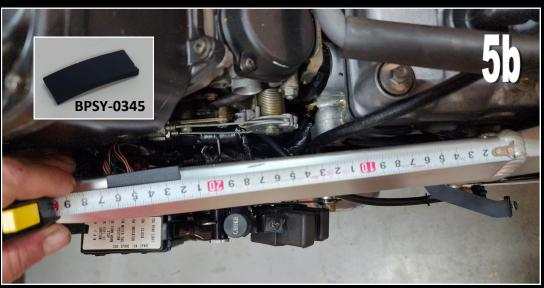
6) The 16956-MT4-000 fuel hose is too long for this application, so we need to cut the hose and also remove some of the plastic shielding.
