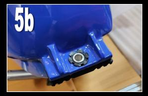
Also fit the BPSY-0345 Rubber, Tank, Side to the frame. These are held with double sided tape. Note the position relative to the weld on the frame, but I advise that you fit these first without gluing and adjust if necessary.
