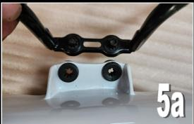
Now fit BPSY-0344 Rubber, Rear Mount, Tank, RC30 and BPSY-0346 Bush, Rear Mount, Tank to the rear of the fuel tank.
