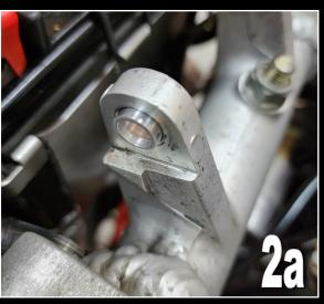
Fit TYLY-0347(W) Tank Mount Rear, RC36-2, RC30 Style (No Fittings) as shown with the bolts provided. Note the direction arrow. This should point to the front of the bike. Try to get the rotation close to the position shown so that minimal adjustment is required when fitting the tank.
