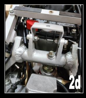
Do not fully tighten at this stage. We will need to adjust when the tank is fitted. **3)** Now prepare the fuel tank for fitting.
