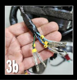
4) The exposed terminals from the blue and green 10P connectors will be directly connected to the extension harness that drives the meter and the running lights. This is described later in this document, but we would like to say that we recommend cutting off the original terminals and fitting normal bullet terminals, as the bullet terminals will be 100% compatible with the terminals on the extension harness and will provide a more secure and reliable connection.
