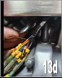
You will notice that wire #4 is not yet connected. This is the 12V for the running lights, so we will connect in a later step. It's advisable to isolate this terminal temporarily to avoid any short circuit during any electrical testing.
