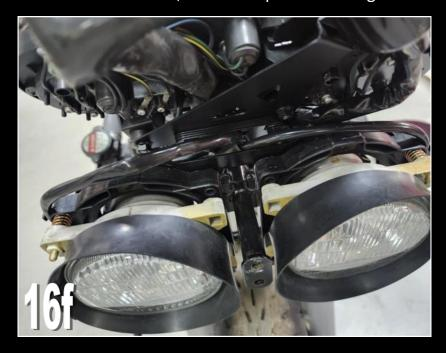
Use the cable tie on the meter stay to secure the wires.
