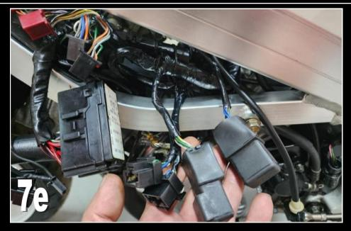
The meter wires and coil wire should be routed from the inside of the lower frame rail and exit on the underside.
