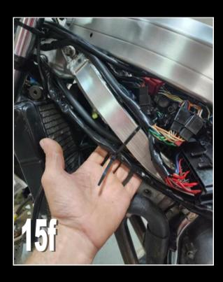
Now run the extension harness on the left side of the meter stay and route it between the meter and the meter stay. Secure to the meter stay with reusable cable tie (provided with meter stay). And finally connect the extension harness and meter stay together and cover up the connectors with the boot.
