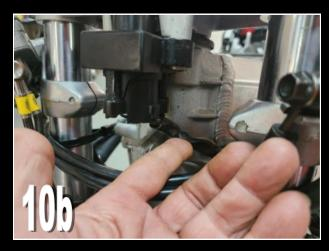
**11)** Route the ignition switch wire on the left side of the fame and connect the plugs as shown
