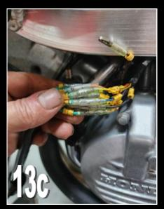
the TYWH-0005 harness does not have the #18 wire for the electronic speedo.
