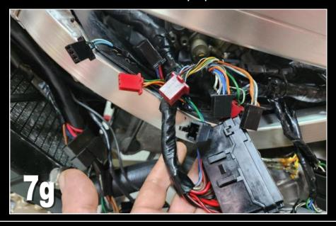
**8)** Locate the 2P fan connector. This needs to run on the inside of the lower frame rail and can be routed under the plastic shield and out to the left of the fame as shown.
