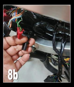
**9)** Moving back to the right hand side of the bike. Route the right hand switch gear wires through the gap between the frame rails and follow the route of the main harness, using the cable tie to secure. Connect the red 9P connector from the switch gear to its mating connectors.
