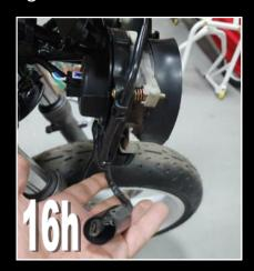
Now run the extension harness on the inside of the fork leg and on the right side of the frame, above the radiator mounting boss. Then it should be routed into the gap between the frame spars and across the front of the carbs. Use the cable tie to secure.
