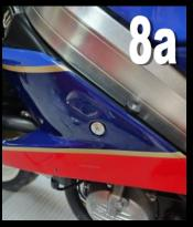
Now to fit the lower cowl. This is quite straight forward but you do need to take care to avoid scratches. I advise to fit the lower from the right hand side of the bike, but first, loosen and move (or remove) the lower left cowl stay, as this can get caught up and possibly scratch the lower if you are not careful and fitting the cowl on your own.
