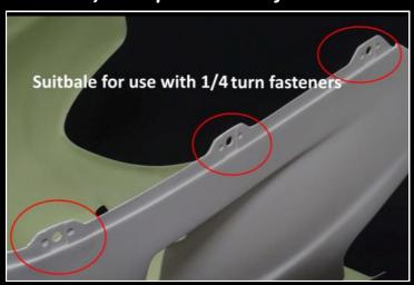
However, for these instructions, we are using the M6 clips. So fit the 6x M6 clips to the mounting tabs.
