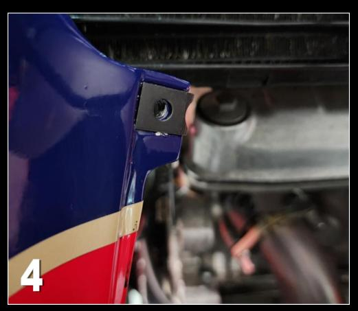
**5)** Now we can move ahead with fitting the upper cowl. The way to do it is to offer into position and fit the front bodywork bolt. Pay attention to making sure that the rubber shield on the headlights stays on the inside of the cowling and does not protrude out of the headlight aperture.
