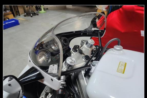
**13)** The final thing to fit is the screen, and if you got this far without too many issues than the screen and molding should be a relatively simple part to fit.
