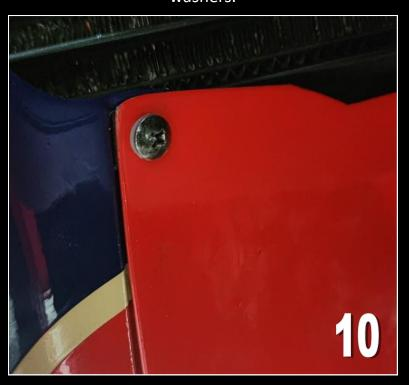
**11)** Fit the bodywork bolt and plastic washer to the lower rear right stay.
