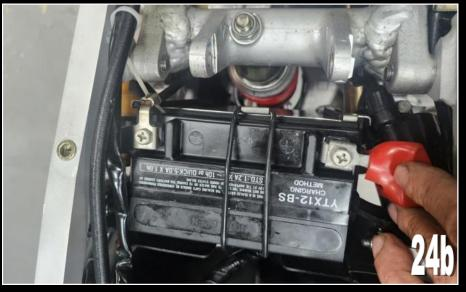
Note that the battery terminal should be connected positive first, then negative. And when disconnecting, remove the negative terminal first.
