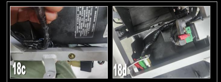
Fully tighten the rear and front undertray hardware to lock it in position.
