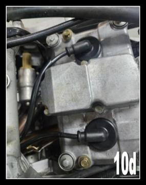
Do not fully tighten the coils up at this stage in case they need a bit of a moving around later.
