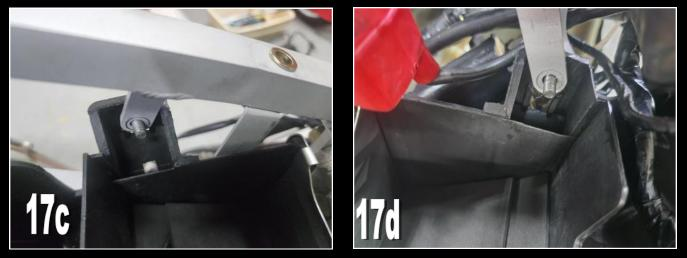
Fit the M6 washers and nuts, but do not tighten yet.
