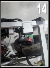
**15)** The harness is routed on the inside of the subframe here and passes under the cross bar. There are three connectors that will be retained in the connector holder at this point.
