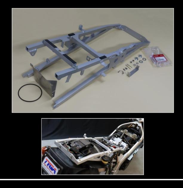
Fitting the TYGA TYLY-0314 subframe is not too difficult. If you managed to remove the standard subframe with ease then the fitting of the TYGA subframe is almost a reversal of that procedure, as we have tried to keep all the components in close to their original position.
