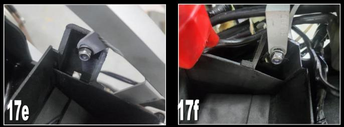
**18)** Now lift the rear end of the undertray up and into position, making sure that all the wiring is routed as intended, and secure to the back plate of the subframe using the original M6 hardware.
