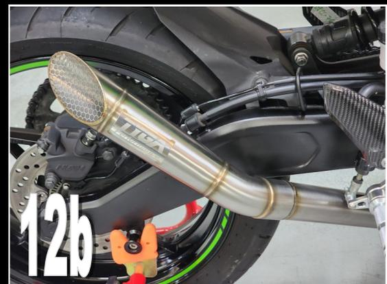
**13)** Now the most important bit of the whole job. Check the routing of the exhaust system from front to back to make sure that all joints are fully home and that you have clearance everywhere. Pay special attention to check that the swingarm can move freely with no chance of bashing into the silencer. Don't be afraid to give the whole system a firm shake around to get the routing perfect. With the multiple sections and slip joints, any small errors can compound.
