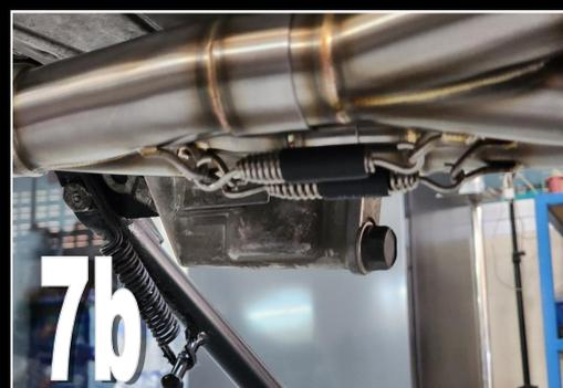
**8)** The next section to fit is the EXPT-8167 tail pipe. Slip the tail pipe onto the secondary collector and give the tail pipe a bit of a twist to get the mounting bush vertical and parallel to the frame mounting face. Secure with the spring on the left side of the pipe. Fit the long M8 bolt through the mounting bush and the frame and spin the M8 nut on finger tight. We'll tighten this up securely as a final attack.
