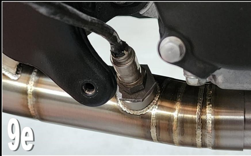
**10)** If you choose to use the OEM M12 lambda sensor, then as mentioned, you'll need to fit the TYWH-0017 wire extension. Simply plugs inline with OEM style connectors.
