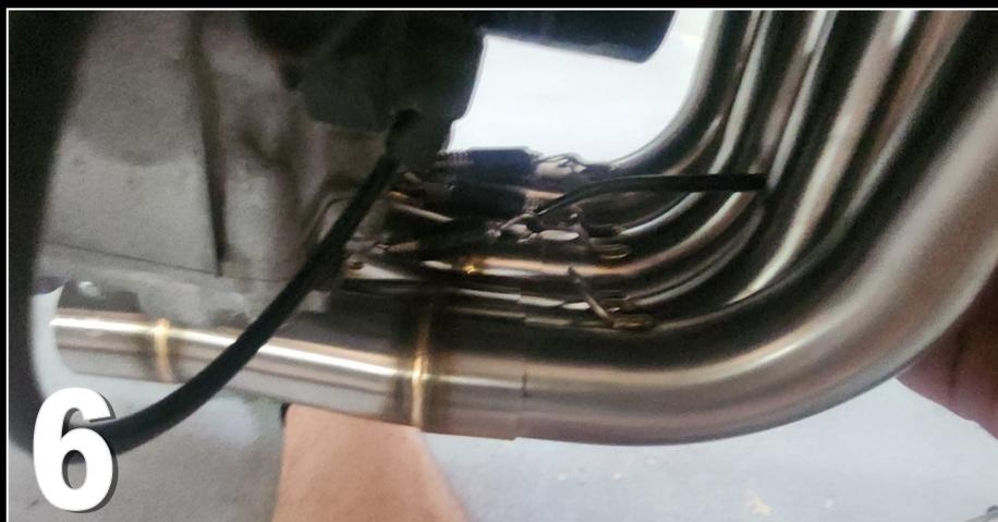
**7)** Now the secondary collector can be fitted. Again, pretty straight forward. Secure to the primary collector with the two springs and give a good wriggle to make sure the collector is fully home.
