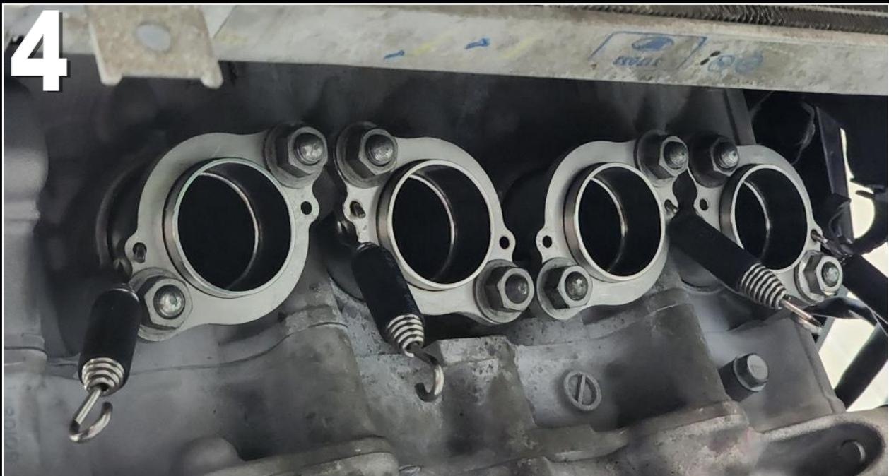
**5)** Onto the headers now. Header #1 EXPT-1167 and #2 EXPT-2167 are joined, as are #3 EXPT-3167 and #4 EXPT-4167. The best plan here is to join them together off the bike and then fit #1 and #2 as an assembly, and then #3 and #4 as an assembly. Slip the headers into the manifolds. They may need a bit of a wriggle to get them fully home. At this point you can fit the springs to stop them sliding out.
