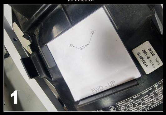
**2)** With the template in position, use a sharp point to make a mark in the plastic. I used my carbide scriber, but just about anything sharp and pointy will do.
