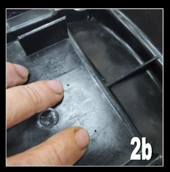
**3)** For a sanity check, offer up the ECU stay and check the hole positions and pitch are correct.
