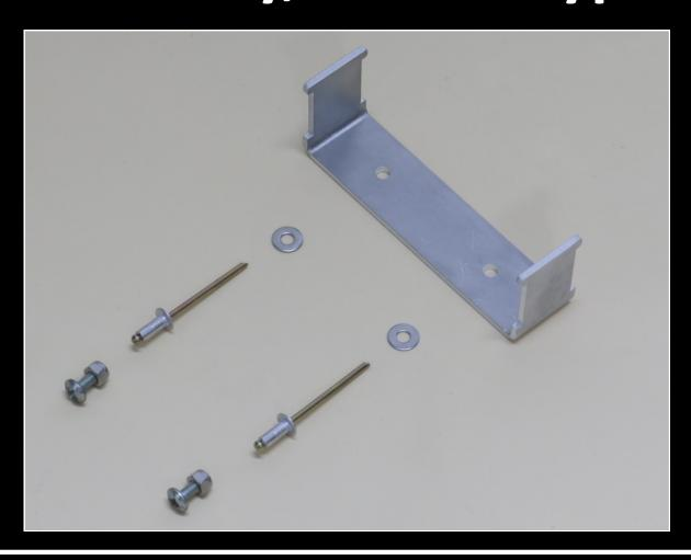
To mount the TYLY-0314X ECU stay, it is required that you drill a couple of small holes in the under tray and secure using either the supplied M3x12 bolts or the rivets.
