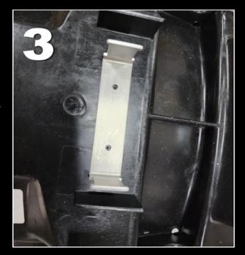
4) Now, drill one hole, and physically locate the ECU stay with a bolt (or rivet) so that you can check that it's going to plan so far.
