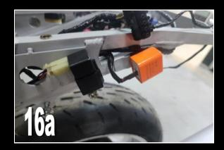
Feed the relay wires through the gaps in the subframe as shown and connect to the main harness. Then they can be tucked out of the way in between the spars. Once the undertray is fitted this will look nice and tidy but can still be accessed if necessary.
