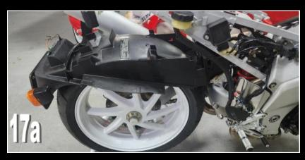
Then you need to lift the front of the undertray up and hook it between the subframe lower left and right spars. The plastic mounts on the undertray are wider than the spars so it takes a bit of a force, pay attention to the heat shield moving into position as it is a tight fit, but it will go through. It is a good idea to protect sharp edges with some painter's tape to avoid scratches.
