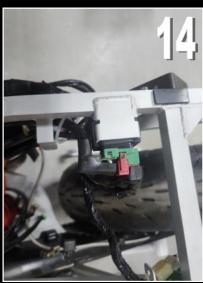
**15)** The harness is routed on the inside of the subframe here and passes under the cross bar. There are three connectors that will be retained in the connector holder at this point.
