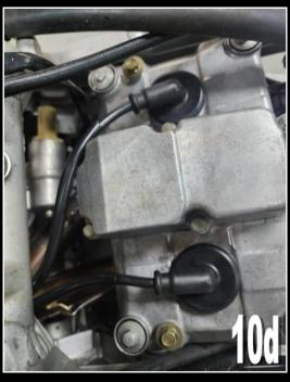
Do not fully tighten the coils up at this stage in case they need a bit of a moving around later.
