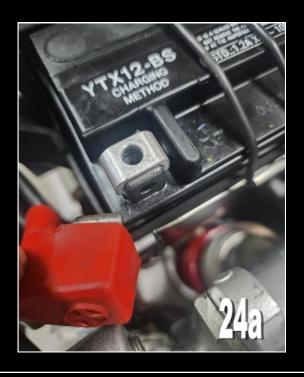
Before connecting the battery terminals, please run though and check the other connectors in the complete harness to be double sure that nothing is going to short circuit. If all the original plugs/connectors are still in place then there shouldn't be any issues, but it's well worth a check.
