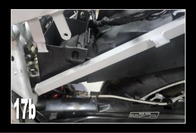
Once in, lift the front into position on the tabs and fit in the original shouldered bolts to retain the undertray in position.
