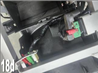
Fully tighten the rear and front undertray hardware to lock it in position.
