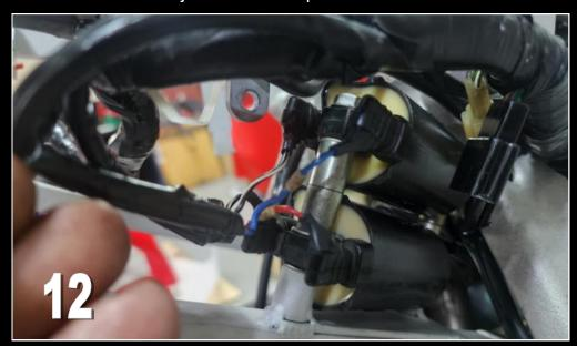
13) Now Bolt on the Regulator/Rectifier tightly and plug in the 5P connector.
