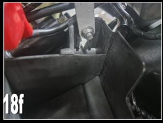
Check that the heat shield mounting tab lines up with the lower right subframe mounting bolt.
