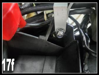
**18)** Now lift the rear end of the undertray up and into position, making sure that all the wiring is routed as intended, and secure to the back plate of the subframe using the original M6 hardware.
