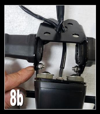
**9)** Now offer the tail tidy up to the bike. First job is to poke the three connectors and wires through the hole where the tail tidy mounts.
