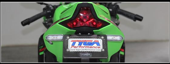
**8)** With the number plate light and the turn signals fitted, the best plan is to fit the main holder back to the assembly and nip up the two M6 bolts just to stop everything from moving around.
