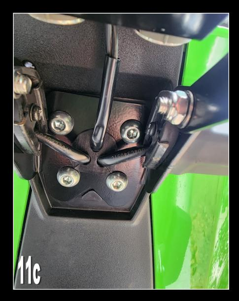
**12)** Before proceeding any further, it is a good time to check that everything is in the correct position and tighten up all the bolts. The tail tidy is very modular and can be configured in several ways, but one thing to try to achieve is to have the reflector in a perfectly vertical orientation.
