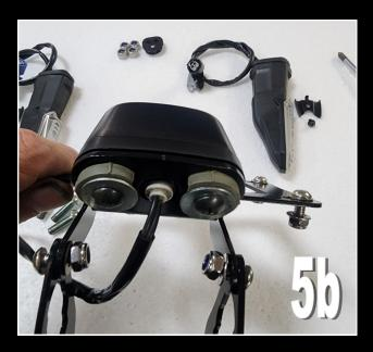
**6)** Next, we'll fit the turn signals. Note that the connectors are different colours. The black connector is the left turn signal, and the blue connector is the right turn signal.
