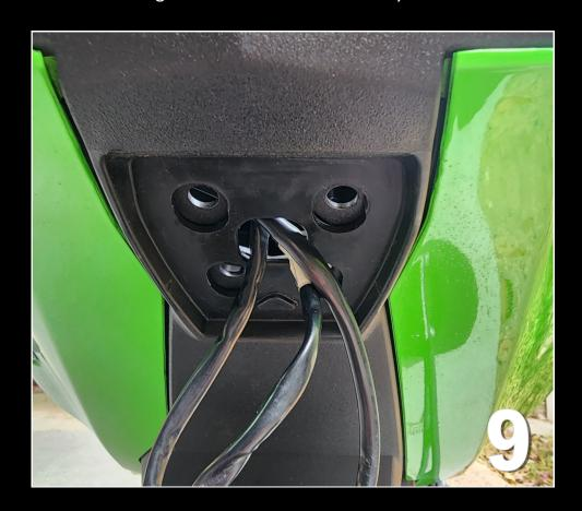
**10)** Use the four M8 button head bolts (original ZX-4R parts) and assemble the tail tidy loosely into position with the M8 Nylok nuts. Don't forget to fit the original wire routing stay as shown.
