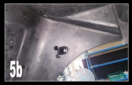
**6)** The next part is a little tricky. You need to fit BPSY-0379B locking plate over the grommet. Offer the plate up at 90 degrees as shown.
