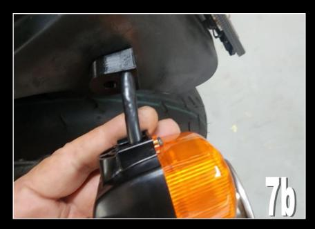
**8)** Fit the BPSY-0382 Bush, followed by the M4x35 machine screw and tighten into the turn signal body.
