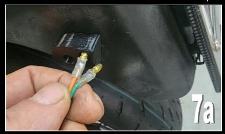
Once through, pull the wiring through all the way.
