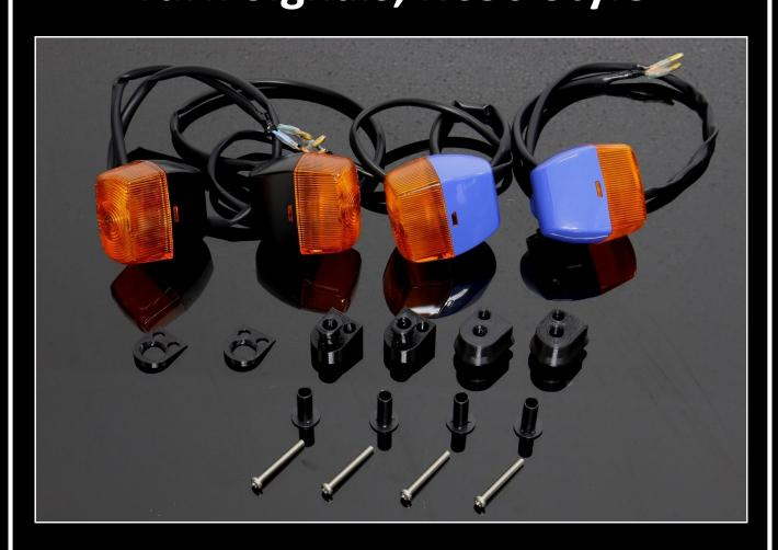
For that authentic RC30 look, we have put together a set of OEM turn signals combined with our own designed 3D printed parts to replicate the style of the RC30 turn signals.
