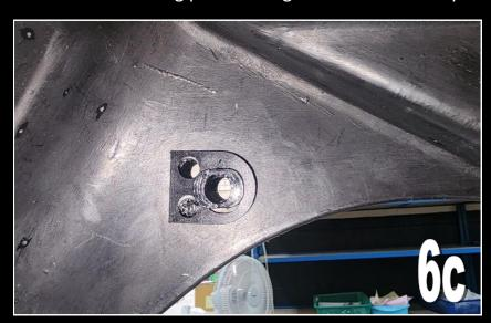
**7)** Now we can thread the turn signal wiring through the hole. Start by offsetting the bullet connectors a little as this will allow easier entry.
