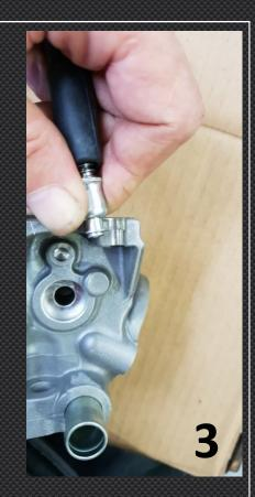
The 'bucket' piece is spring loaded. Pull this back and hook the piece into the slot of the aluminium on the cylinder. The circlip on the end should be on the underside and the bucket on top, as shown in picture 4 This then preloads the spring on the return (close) cable.
