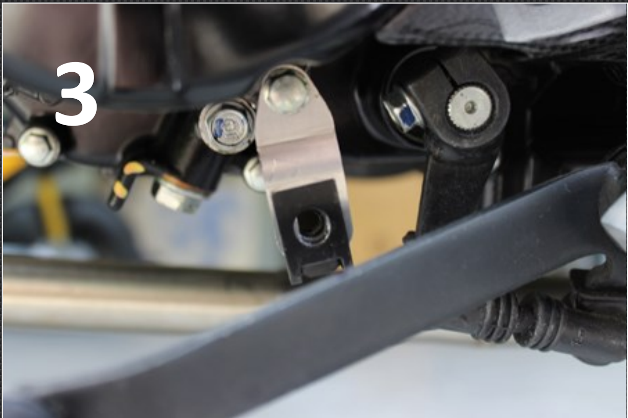
3) Rear left stay mounts on the side of the engine using the existing M6 bolt as shown in the photo
