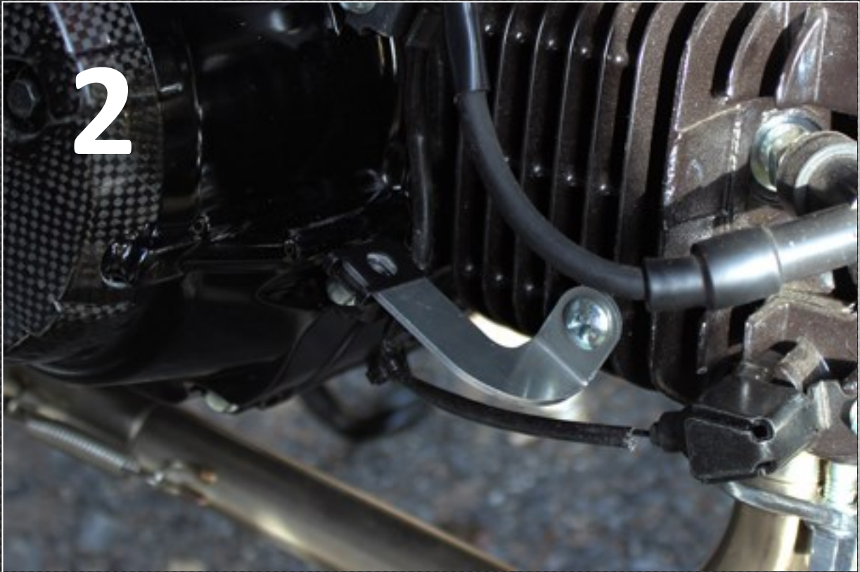
2) Front right is supplied with M6 bolt and mounts on the threaded hole on the cylinder. See photo for orientation
