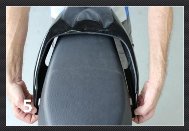
5. Hold each front part of the seat cowling either side and pull them past the mounting stays. Be careful not to scratch the paint.
