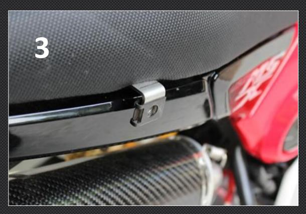
3. Put the M6 clips on the stays with the closed end pointing backwards.
