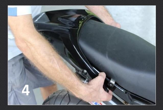
4. Offer up the seat cowling from the rear of the bike so the securing tab engaged the rear of the seat pad when it is fully in position.
