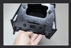
The MSX125SF has a belly pipe as standard, so for fitting the TYGA High level pipe it is necessary to modify the standard rear fender to fit the stay (BPSY-0175 / BPSY-0177), which is used to secure the silencer in position.
