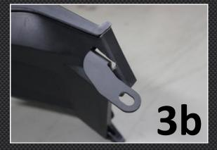
Offer up BPSY-0175/0177 to check fit and clearance. And trim any interference as necessary.
