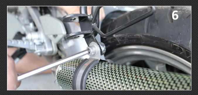
7) Finally, turn your attention again to the belly of the exhaust and make sure everything is sitting where it needs to. For US model Cup bikes, the bracket is slightly different and sits more inboard. We provide a bush to install, to allow the exhaust to sit in the correct position. You can see it installed in the photo bellow. Also note that due to loosening of the bracket, the stay which holds the rear left position of the fairing may need adjusting when the bodywork is installed later.
