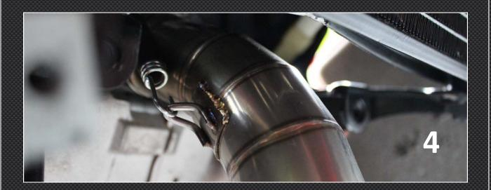
flange and the internal hole in the silencer where the exhaust chamber mounts. You will notice there is an 'O' ring in the silencer but extra sealant will also act as a lubricant until it sets aiding installation. Once the silencer is in place, install using the three bolts provided, putting all in finger tight first and tightening once they have all been installed.
