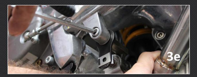
4) Now would be a good time to install the springs on the header. These are installed just the same way as the stock ones and again you will need either a tool or piece of wire and pliers.
