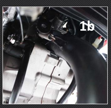
Turn your attention to the belly section of the chamber and you will see it is held to the bracket which in turn is held on to the foot peg hanger. Remove the bolt from the bracket so the chamber is free in this position while holding the exhaust system. Next, remove the loosened bolt from the silencer and remove the complete exhaust system from the bike.
