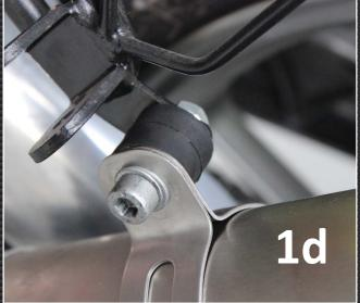
Finally, you need to remove the two bolts holding the manifold to the cylinder. After removal of the bolts, you can then remove the two exhaust spring brackets, the stock manifold and the gasket in that order. You will need to re-use the two exhaust stud nuts and the gasket. The bike is now ready for the TYGA Exhaust system.
