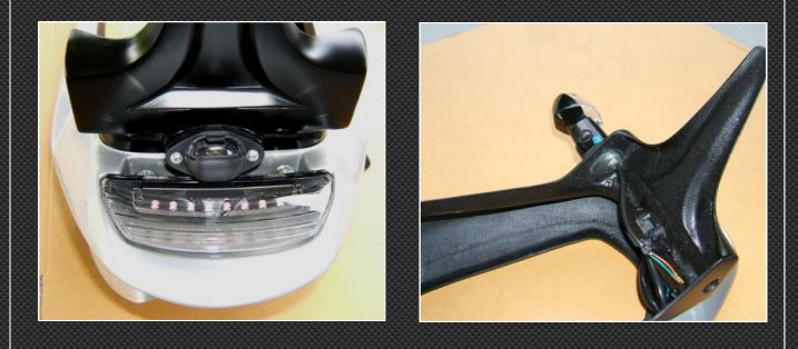
5. The next job is to connect the seat lock mechanism. To do this, thread the barrel from the outside to the inside of the seat unit as shown in the photo below. It maybe a bit tight to get the clip in the grooves in the barrel. In this case, you can remove the rubber from between the barrel and the outside of the seat cowling to give extra clearance. You then need to install the cable by slotting it in the cup and clipping it in the cable bracket.
