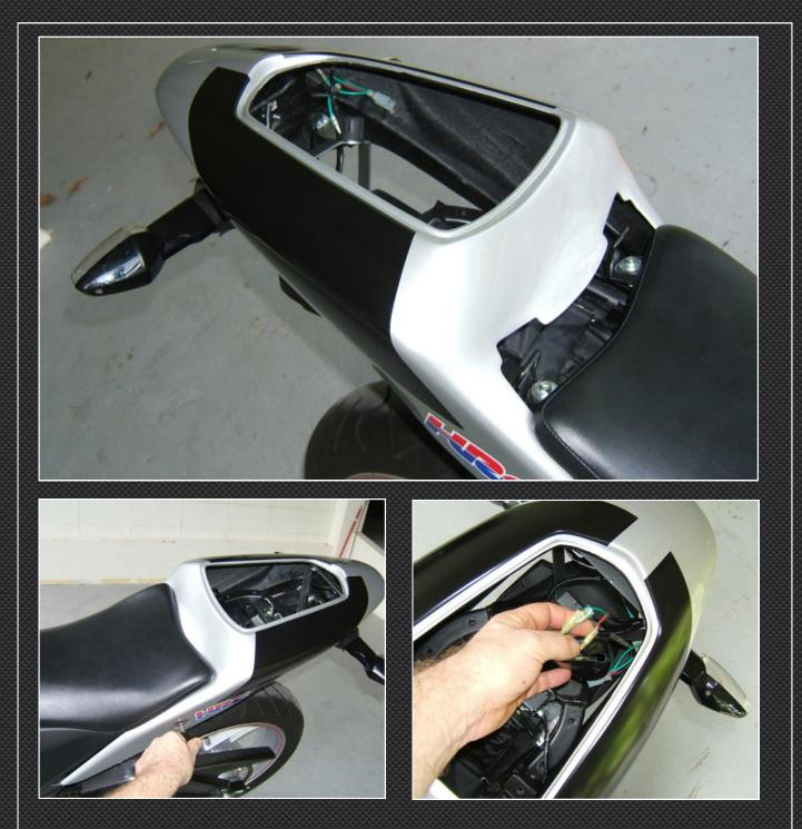
7. Once you have landed the seat cowling in position, pop the inserts into the rubber bushes at the front of the seat cowling. Be careful the inserts don't dislodge the rubbers and push them through. Note there is no other direct mounting point for the seat cowling. It is held in place at the rear by the seat cover and the seat stay cushions. Also check the latch mechanism operates properly when you turn the key. Connect wiring and test.
