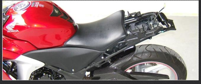
3. Put the rubber cushions in the seat stay as shown in the photo below and mount the undertray in position. You need to thread the bolt from underneath the undertray and into the frame until it is tight. The end of the bolt should now be sticking up out of the frame. Put the seat stay over the bolt and tighten using the nut provided
