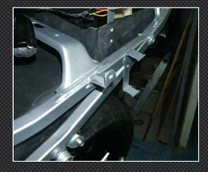
Once the undertray is in place, it is necessary to make some modifications to the subframe in three places.
