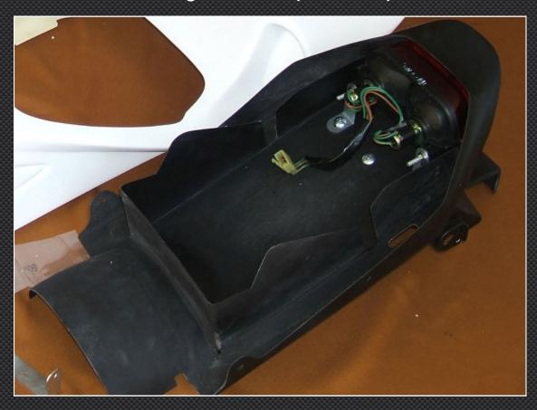
This replaces the stock item and fits using the bolts provided. Make sure first that you route the various wiring components as you go to make sure the wires don't get pinched or damaged when you put the rear fender in place.
