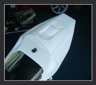
Now, turn your attention to the front two hooks and check they properly engage when the latch is operated. It is easential that the latch does not stick because the passenger seat cover can not be removed once the rear fender is installed. Also, if it does not engage on the hooks, it may fall off the bike.
