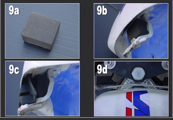
10. Next, the rear of the tank needs to be secured. If not already done, remove rear tank rubber. Slide the front of the tank into position and place the nylon spacer block between the tank and the subframe. Line up the rear hole of the two on the subframe and secure the tank in position using the M8 bolt and washer. Refit the fuel and vacuum hoses. The tank is now done.
