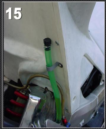
15. Fit the HRC rear brake reservoir kit. Remove the stock brake reservoir by doing the following.Clamp the hose flat to prevent flow at as low a position as possible.
