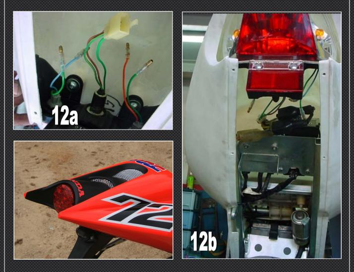
13. The subframe stays can now be fitted. There are two inserts in the underside of the subframe. The stays are secured to these by way of the bolts provided and should be fitted so that they slope outwards to meet the under portion of the seat cowling. Mark and drill the seat cowling in the correct place and secure the seat cowling to the stays using the M5 bolts provided. This will reduce the amount of vibration on the seat cowling when riding.
