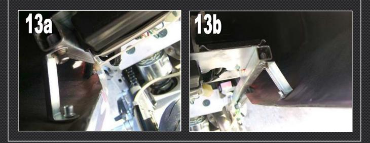
14. The undertray can now be fitted. Slide the front into position and arch the rear up past the reflector on the taillight and into position. Loosely fit all M4X10 mounting bolts and check for alignment again. Fine tune the tail cowl alignment if necessary and secure tightly the undertray bolts.
