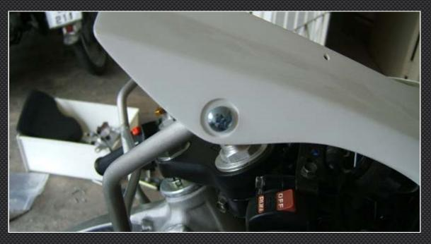
Next fit the side cowlings in position. There are four securing bolts to the front fairing for each side. Two on the outside and one each on the console and inside near the front air duct. Secure these in place.
