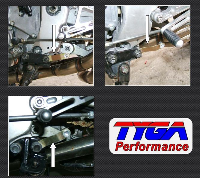
On the right side, the lower stay fits in the bottom foot peg hanger position, remove the hanger and sandwich the right lower stay between the frame and the bush or hanger if there is no bush. To keep hanger square with bike, place washer provided in the upper hanger position. Do not tighten yet because you may need to adjust stay later.
