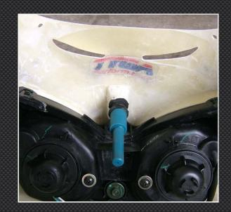
Now, from the front of the bike, slip the upper into position. Once close to the bike, the cowl all the remaining electrics can be connected.
