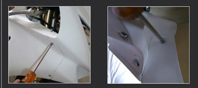
Check the alignment of the side mounting holes of the cowling with the side stays on the bike. On the NC30, don't be afraid to tweak the stay into position. On the NC35, rotate the stays into position as necessary, Secure fasteners once the stays are in position.
