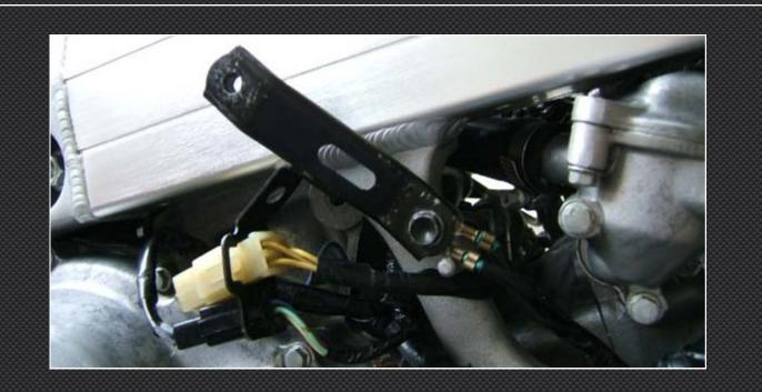
Finally, note position of console stays, mark in correct position and drill to accept M4 bolts provided. This is quite difficult, but the stays are adjustable so you can make minor adjustments if necessary
