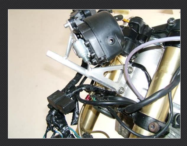
Fitting RC211V Style Upper Stay (TYLY-0020 and TYLY-0021) and console stays Replace the stock stay with TYLY-0020 (NC35) or TYLY-0022 (NC30). Offer up the stay into position.
