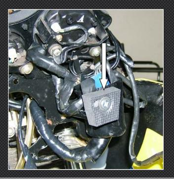
On the NC35, it is secured to the RC211V Meter stay by way of a rubber front stay and nylon bush that slips inside the main tube of the meter stay. Thread this into position on the front of the fairing before attempting to fit the front fairing to the bike.
