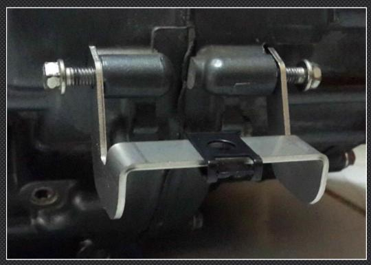
Do all the bolts up finger tight at first and check the position and clearance of the belly pan. Once you're happy, do it all up tight.
