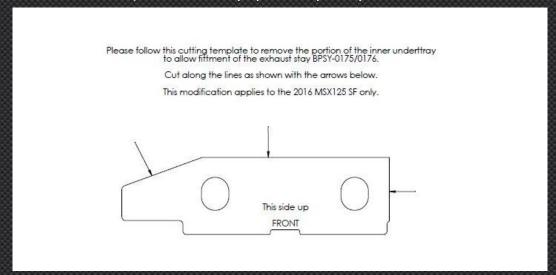
2) Offer up template to part and mark off as necessary. Use tape or scribe a line.
