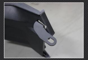
Offer up BPSY-0175/0177 to check fit and clearance. And trim any interference as necessary.
