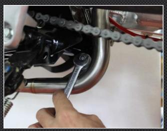
4) We are now ready to install the final section. This slides onto EXPT-0036 and one of two types are supplied in the kit, EXPT-0037 for most applications and EXPT-0065 which is slightly longer for systems using the oval silencers on the second generation MSX125SF Grom. In all other respects the two types of final sections are the same and are secured by springs to the intermediate section.
