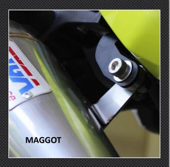
For all models, it is important to ensure that there is clearance with bodywork and that the silencer is not under any stress on the mounting points. If it is, there is a good chance that the installation is not correct. Repeat steps above and try again. Once you are happy with the position of the exhaust, secure tightly all mounting points of the exhaust including the exhaust stud nuts, the frame mount and the silencer stay.
