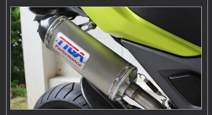
1) After removing the Honda exhaust, you will need to re-use the nuts for the exhaust pipe on the engine and the bolt where the exhaust mounts to the frame on the right hand side. All the other components are supplied with the replacement exhaust. First install the header section (EXPT-0035). Install this loosely using the Honda exhaust stud nuts.
