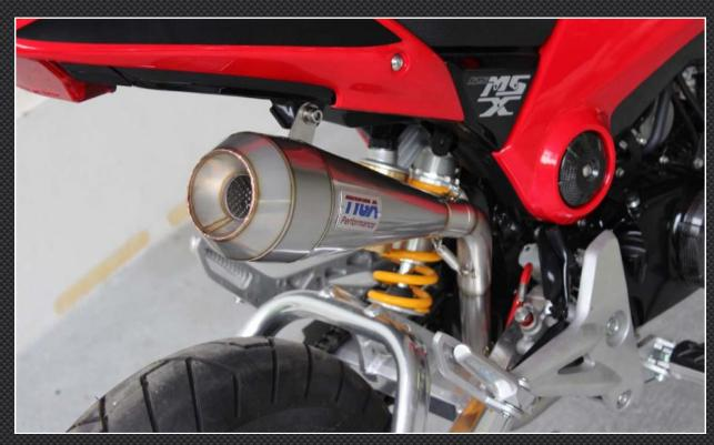
For second generation bikes, the oval silencer fits to the silencer stay BPSY-0177 on the outside as shown in the photo. For the maggot, it can be installed on the inside of the stay BPSY-0175 and spaced using the aluminium spacer provided. Note a longer bolt is supplied for this reason.
