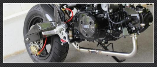
b) For earlier types, which can be identified as not having the lightening hole in the exhaust mounting lug, they secure inboard of the frame as shown here. To install them, thread the Honda mounting bolt all the way through the frame first and tighten. Then slide the intermediate section of the TYGA system onto the bolt from the inside of the frame as shown in the photo and secure using the nut and washer provided with the exhaust system. Now move on to 4.
