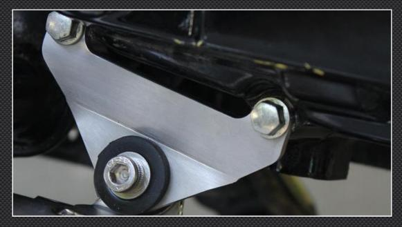
3) Do up the header pipe stud nuts, finger tight only at this point.
