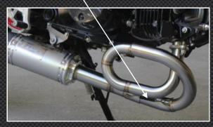
6) Make sure that there is clearance on any bodywork and other components and tighten up the exhaust studs and the bolt for the exhaust stay. Finally, tighten the small M4 locking screw at the silencer slip on joint. You are now ready to ride.
