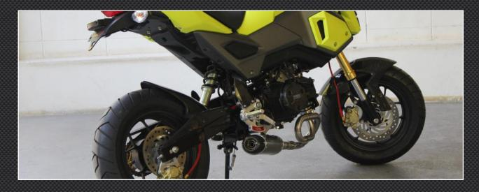
4) Slide the silencer into position and insert the bolt. Note that the bolt is inserted from outside towards the centreline of the bike in the order of:
