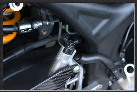
Now remove the master cylinder from the step kit and continue as normal to fit the step kit to the bike. With the main step assembly fitted, now fit the master cylinder loosely. Attach the "End B" of the replacement hose to the brake caliper as shown below.
