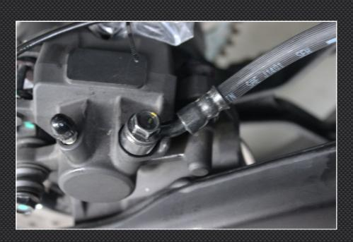
Now secure the master cylinder tightly to the step hanger, and then tighten the banjo bolts, being sure that there's no hose kinking.
