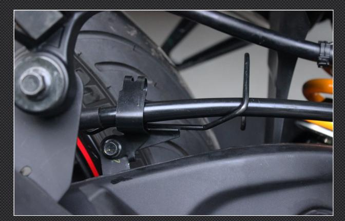
Check rear brake operation and bleed as necessary. Finally, check rear brake light operation and adjust as required.
