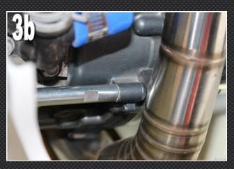
**4)** Attach the lower left rear stay as shown. The M8 bolt on the frame should be screwed through, and then the stay fitted and nipped up with the nyloc nut. Do not fully tighten at this stage.
