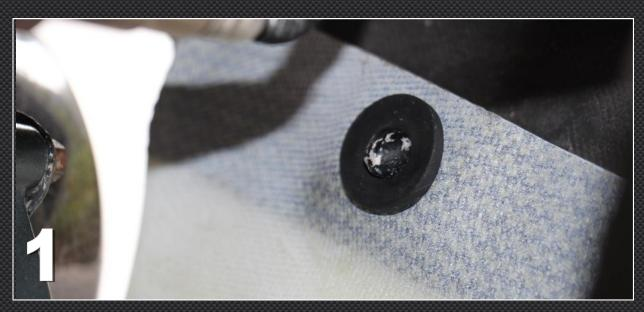
**2)** If not already fitted prior to shipping, fit the drain hole bung to the hole in the Belly-Pan
