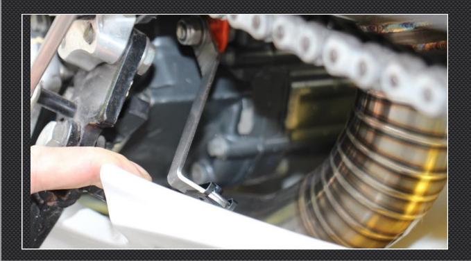
**5)** The rear right stay (with M6 insert) should be secured to the step kit as shown. Just finger tight at this stage.
