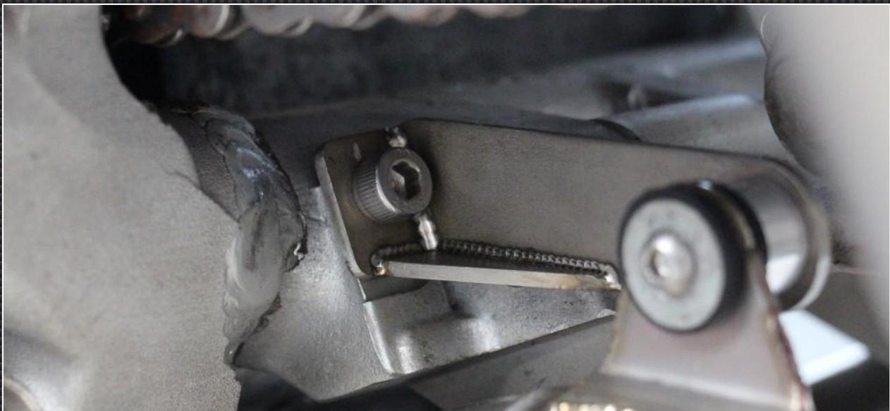
**15)** Now take a good look all around and check for interference issues with the frame, swingarm, cowling etc. The routing of the pipe does have a little adjustability by a bit of twisting here and there.
