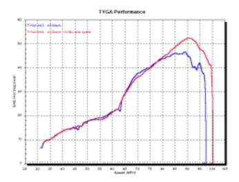
2. TYGA SS pipes with aluminium silencers. Shown below compared to stock and wire splice.
