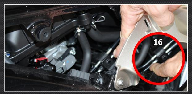
**16)** Pop out the bottom of the two lines from the holder to allow the line some freedom of movement.
