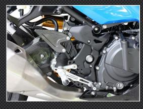
Designed in-house by TYGA Performance using the latest CAD/CAM software, these CNC machine-made step kits are made from top quality aircraft grade aluminium. Complete with carbon heel guards on left and right hanger.
