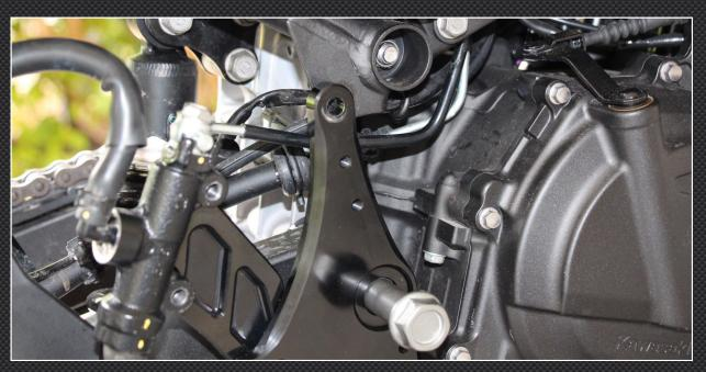
19) Loosely fit the M8 button head bolt (provided) into the top hole of the main plate.20) Loosely refit the M10 bolt into the lower hole of the main plate, followed by lower fairing mount stay and 33mm bush. The fairing mount stay is located between the main plate and bush.
