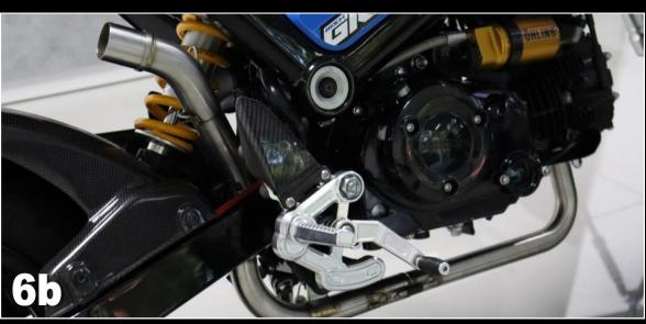
**7)** Fit your silencer of choice, secured by the two springs to EXPT-0083 and then wriggle the silencer into position with the stay. The silencer mounting tab is (by default) fitted on the inside of the grommet in the BPSY-0304 stay. Nip up the M6 button head.
