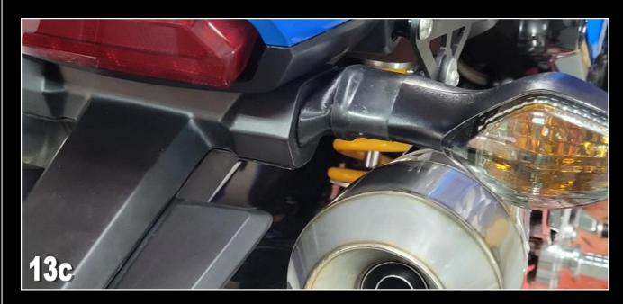
**14)** Alternative spacer BPSY-0308 can be used if aftermarket turn signal indicators such as BPLT-0030 Slim Style LED turn signals are installed.
