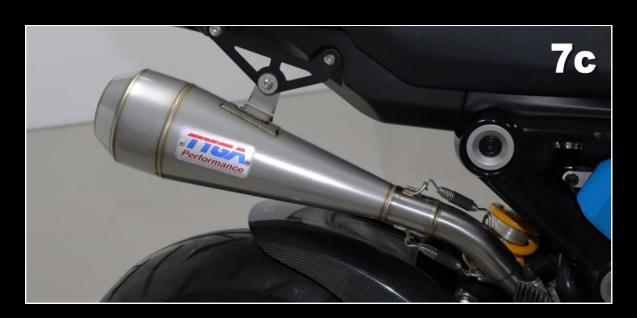
8) Check that the pipe is clear and has no interference and that the silencer is sitting in the correct position and then tighten everything up, starting with the M8 dome nuts on the header, then the frame mount and finally the silencer mount and silencer stay.
