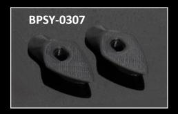
These locate the indicators a little wider and further forward than stock, giving extra clearance from the silencer. Fitting requires that you remove the inner plastic cover from the rear fender by removing 4x screws and an M6 bolt. The cover can now be removed.
