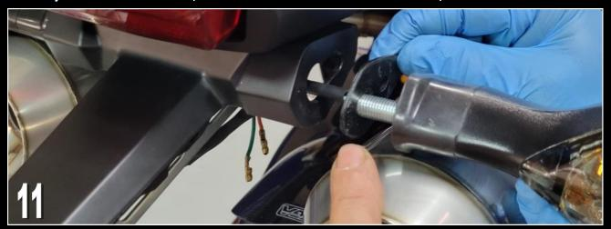
**12)** Feed the indicator wires through the BPSY-0307 spacer as shown and allow it to locate.
