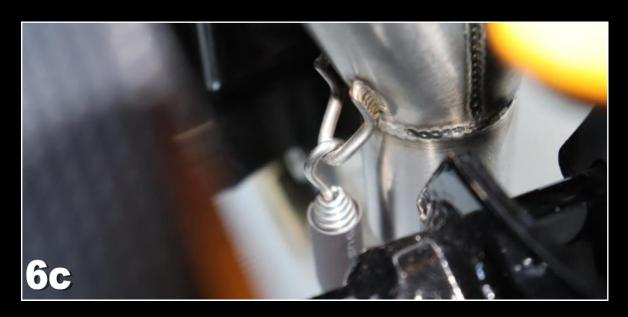
7) The two final sections, EXPT-0085 and EXPT-0086 can now be fitted. Again, hooking the springs onto these sections first makes the job just a little easier. Slip then onto the collector and secure with the springs. The springs can be a little tricky to fit, but the best plan is to fit the left side spring from the right side of the bike and then the opposite for the right side spring.
