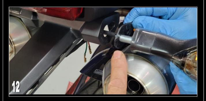
**13)** Feed the indicator wires through the BPSY-0307 spacer as shown and allow it to locate
