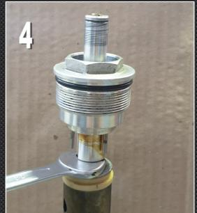
**4)** Pull down the preload spacer with a bar in one of the holes in the preload spacer, and you can now jam a 14mm wrench onto the rebound damper locknut. This will hold the preload spacer down.
