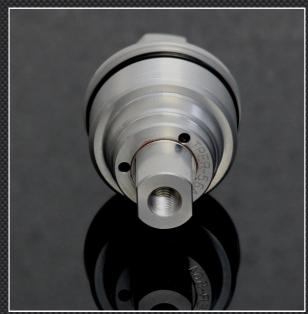
Please note that you should always assemble the caps onto the fork with the fork at full extension. So this means either with the forks removed from the bike, or if the forks are still in the bike then the front end should be off the ground so that the forks are fully extended.
