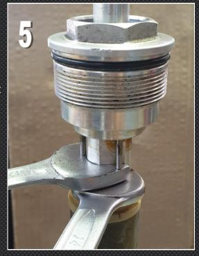
**6)** Use the 14mm wrench to help keep the spring compressed and wind off the fork cap assembly from the damper rod. Now pull the fork cap off completely. The rebound adjuster rod will come out together with the fork cap assembly.
