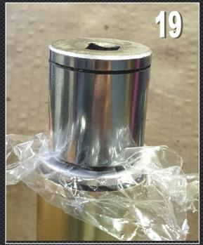
**19)** Fit the fork cap assembly back into the top of the fork. I use a piece of plastic bag (or similar) here to help to protect the components. You don't want to put a ding in your brand new parts
