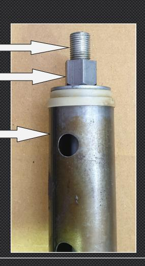
1) Wind down the preload adjuster a few turns and remove the circlip, if it's still there. It wasn't on my sample fork
