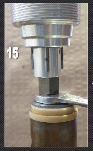
**15)** Now wind up the lock nut again the rebound adjuster holder. Again, just nip it up finger tight at this stage. Do not use any tools to tighten at this stage or you could cause damage to the rebound damper needle
