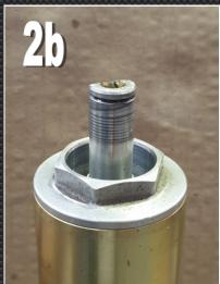
**2)** With the circlip removed, now wind the preload adjuster completely off.
