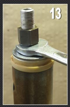
**14)** Insert the rebound adjuster rod into the damper rod and screw the assembly onto the damper rod. You will feel it go tight when the rebound damper needle makes contact deep inside the fork. You only need to be finger tight here
