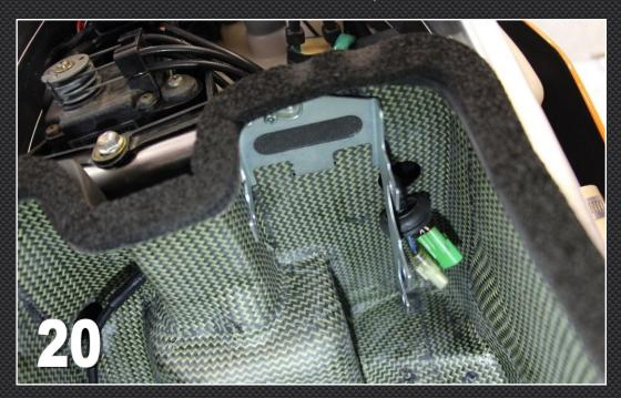
**20)** At this point you can fit the solenoid/TPS grommet into the air box hole, but leave the other grommets out for the time being.
