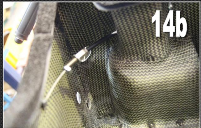
**15)** Push the air box down further, just make sure that you guide the transmission breather hose up through the hole in the sealing rubber so that it doesn't kink or jam. Let the air box rest a little way above the engine.
