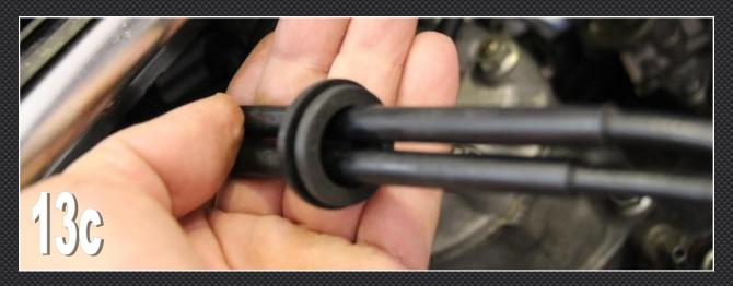
**13d)** Choke cable in hole H using single hole 16mm. grommet.
