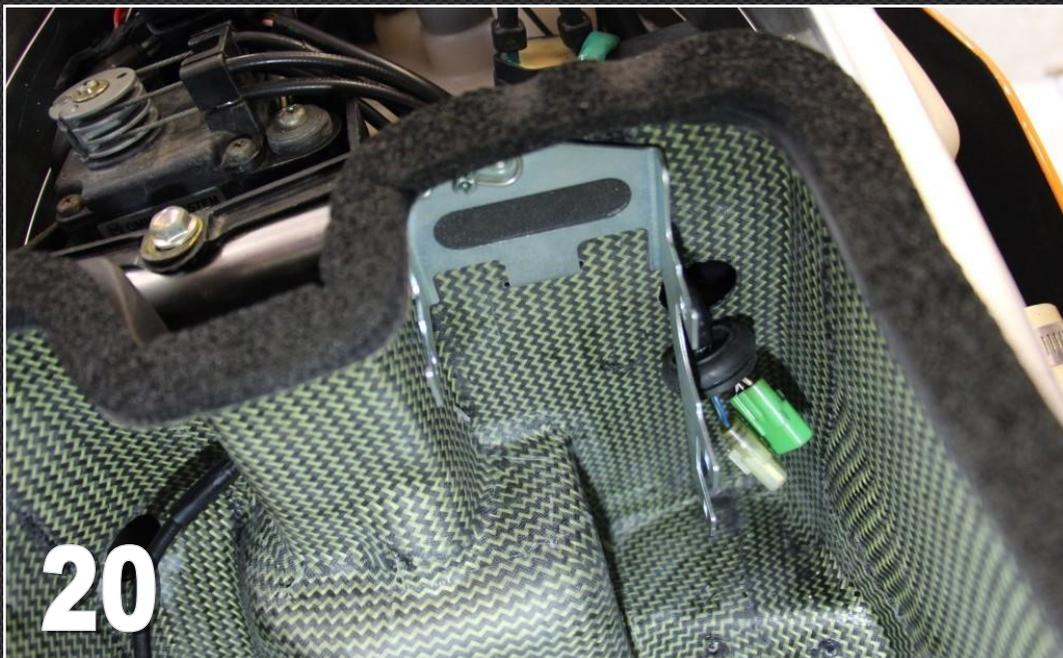
**20)** At this point you can fit the solenoid/TPS grommet into the air box hole, but leave the other grommets out for the time being.
