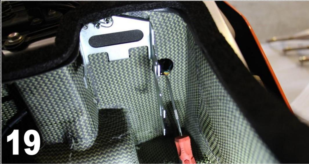
Note here that the air solenoid stay is already pre-fitted to the air box, but if it is getting in the way then feel free to remove the single quick fastener and then remove the stay. You can re-fit this at any time.
