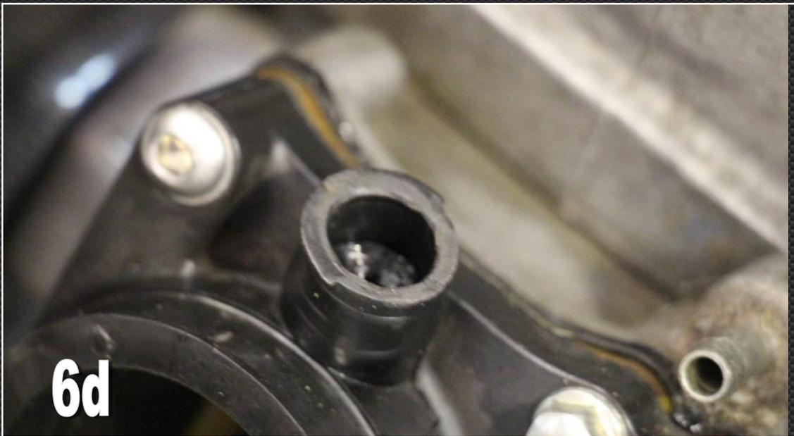
7) Remove the 4x outside M6 bolts from the insulator and replace with the 4x M6x30 button head bolts.
