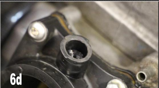
**7)** Remove the <u>4x outside M6</u> bolts from the insulator and replace with the 4x M6x30 button head bolts.
