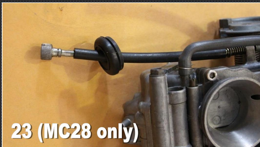
**24)** Now fit the throttle cables and 2T oil pump cables to the carbs. It's usually easier to fit the throttle cables and 2T oil pump cable prior to actually popping the carbs into the insulator as you can move the carbs around a little.
