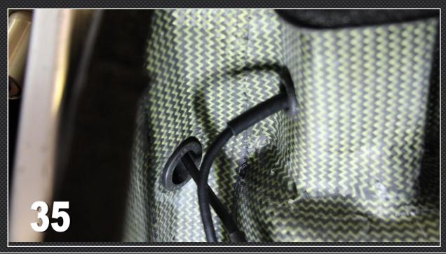
**36)** Connect the choke cable and fit the 16mm. grommet into hole H.
