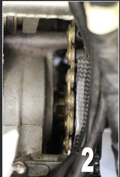
**3)** Make sure the wiring harness is running below the main left side frame rail at the front and then above the casting for the rear shock as shown in the photo to get clearance with the air box. The air box is relieved to provide adequate clearance for a street harness.
