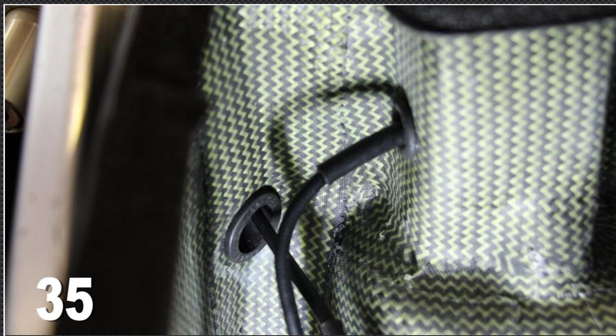
**36)** Connect the choke cable and fit the 16mm. grommet into hole H.
