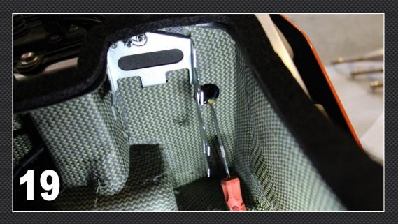
Note here that the air solenoid stay is already pre-fitted to the air box, but if it is getting in the way then feel free to remove the single quick fastener and then remove the stay. You can re-fit this at any time.
