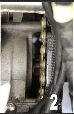
**3)** Make sure the wiring harness is running below the main left side frame rail at the front and then above the casting for the rear shock as shown in the photo to get clearance with the air box. The air box is relieved to provide adequate clearance for a street harness.
