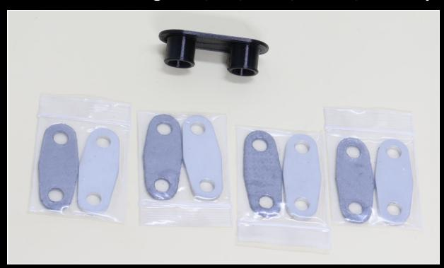
These blanking plates are used to blank off the PAIR Valve holes into the exhaust ports after removal of the complete PAIR valve system.
